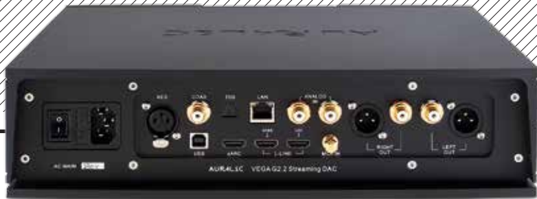
ABOVE: Digital inputs on AES, coaxial and optical (192kHz/24-bit and DSD64 over DoP) are joined by wired LAN, USB-B and Auralic Lightning Link ports (384kHz/32-bit and DSD512) plus an external clock input. Line inputs (on RCAs) sit alongside fixed/variable preamp outputs on XLRs (balanced) and RCAs
